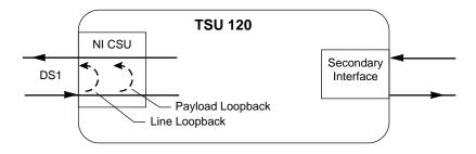
Figure 7-2. Network Loopback Tests
